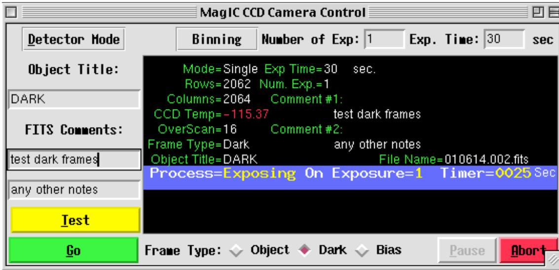
Once the exposure is complete the Process bar will indicate Reading until the file is readout and the system is ready for the next action.
