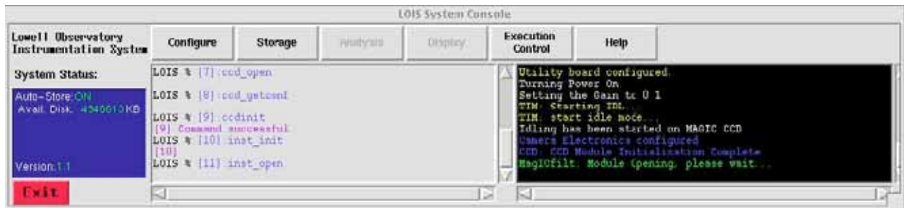
Figure 3. LOIS System Console. The log screen on the right-hand side tells the user what the instrument is doing.
