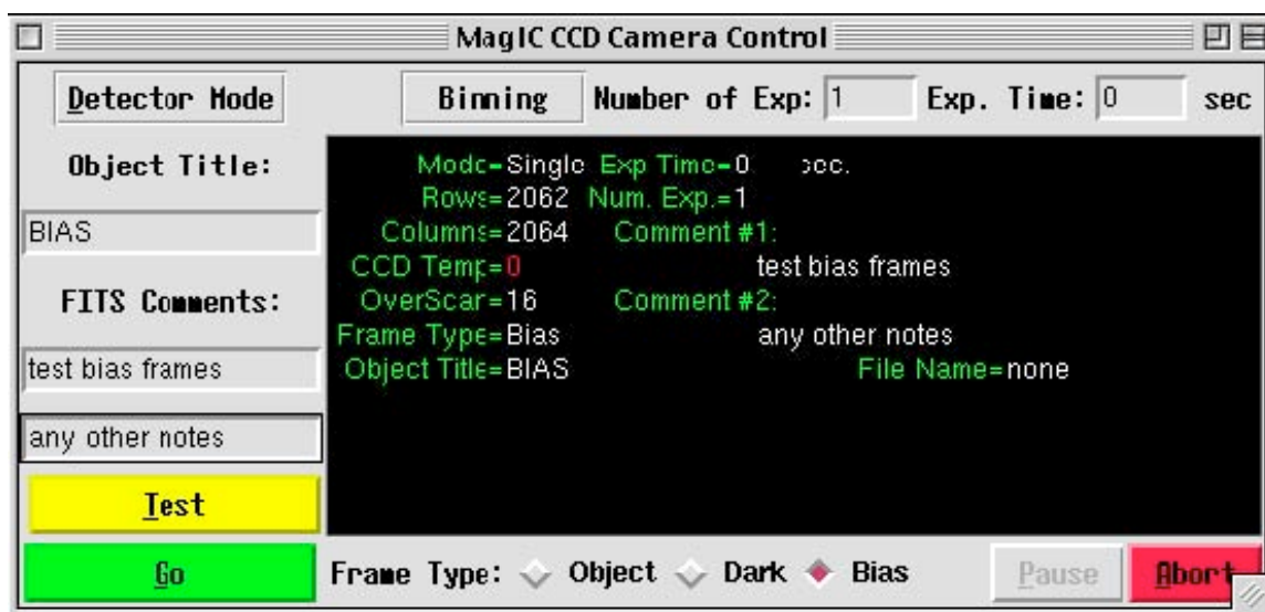
Figure 7. MagIC CCD Camera Control module. This module is where the observer defines the requirements for the observations: number of exposures, exposure times, object title, type of image (object, dark, bias), binning, detector mode and comments. It is also the module from which the observer starts the camera collecting data by selecting either the "test" or "go" buttons.
