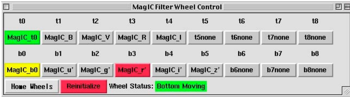
Figure 11. MagIC Filter Wheel Control, status during selection of new filter and motion of filter wheel. Yellow indicates the filter that the wheel is moving from, the red filter name indicates that is the filter the wheel is moving to.
