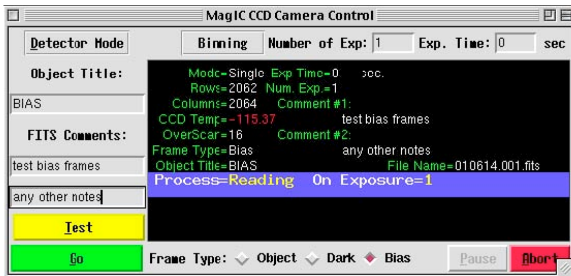
Figure 9. MagIC CCD Camera Control status of readout progress.
