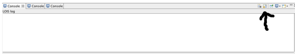
Figure 9: Console log window. Clicking lock button (giant arrow) allows you to stop automatic scrolling of the console log. This button is very handy if you want to look through the log for triggering messages while you are imaging.
